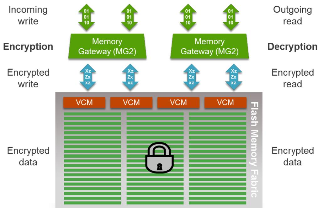
Figure 6: vMOS Encryption ensures complete protection of all data written to Violin Systems Flash Arrays
