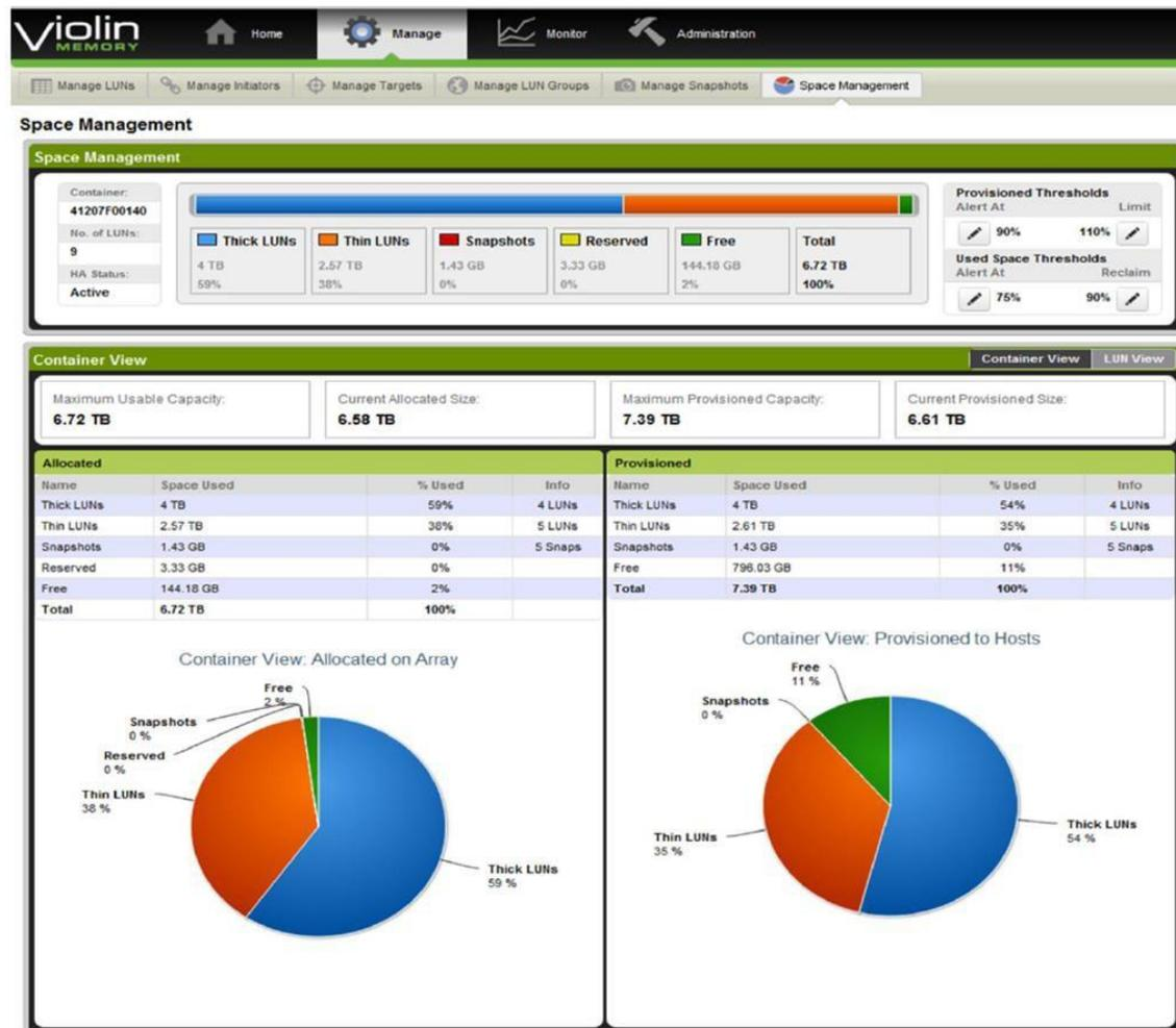
Figure 9: vMOS WebUI provides easy administration and management of thin provisioned LUNs
