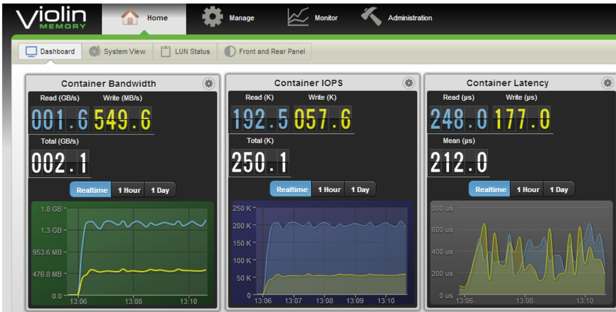
Figure 4: Violin GUI screen capture running SLOB2 workload on a single server attached to one Violin array
